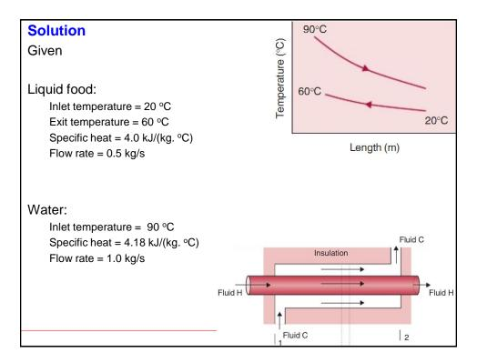
(a) Using simple heat balance equation:
