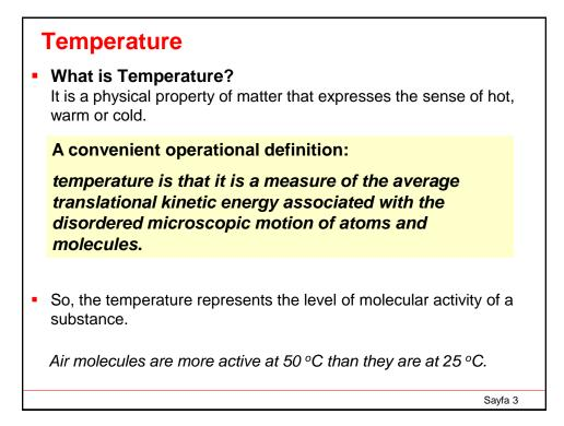
When a high temperature object is placed in contact with a low temperature object, then energy will flow from the high temperature object to the lower temperature object, and they will approach an equilibrium temperature.
