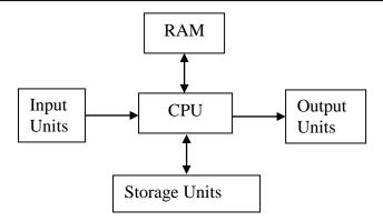
Figure 1.1: Block diagram for the hardware parts of a digital computer
