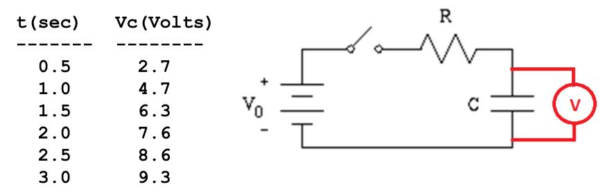
where *t* is time and *Vc* is potential difference the across the capacitor. Using least square fitting method, determine the time constant of the circuit if  $V_0 = 12$  V.
