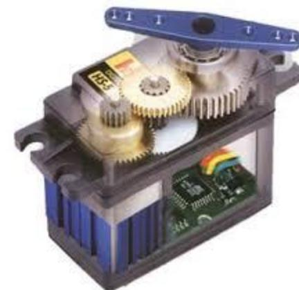
A servomotor is a rotary actuator that allows for precise control of angular position, velocity and acceleration.
