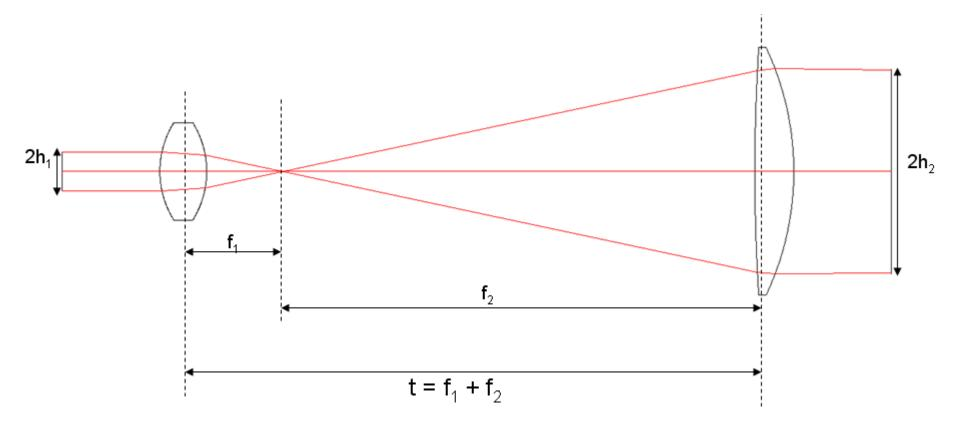
$$m = f_2/f_1 = R_2/R_1 = h_2/h_1$$
