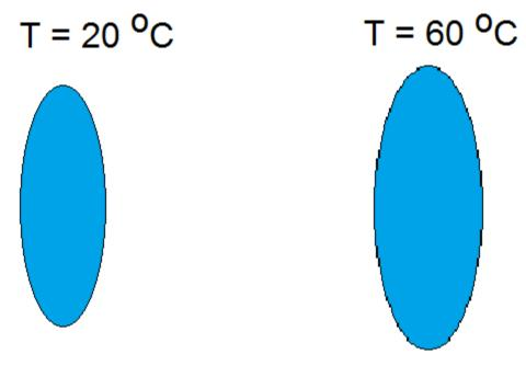
Exaggerated thermal expansion of a lens
