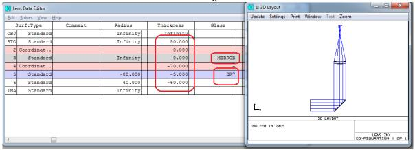
**Ex3.** For two spherical mirrors, derive Cassegrain Telescope Design Equations via paraxial ray tracing equations.  $\frac{1}{f} = \frac{1}{f_1} + \frac{1}{f_2} - \frac{d}{f_1 f_2} \text{ and } d + b = \left(1 - \frac{d}{f_1}\right)f$
