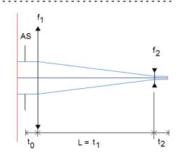
**Ex5.** Perform paraxial and real ray tracing for a given ray in figure. Determine value of x for each case and compare your results. Assume that radius of curvature of first lens is  $R_1 = 100$  mm and of second surface is  $R_2 = -100$  mm.
