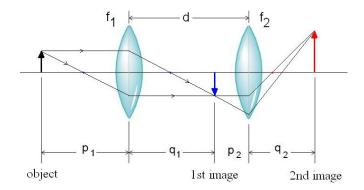
**Ex2.** For the system given in Ex1, find EFL, BFL and FFL of the system if  $f_1 = -30$  mm,  $f_2 = +20$  mm and d = 10 mm. Implement your solution in Zemax and compare your results.
