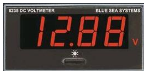
Fig A2: Digital voltmeter having a maximum uncertainty of \pm 0.005 \text{ V} for this reading. So the value and its error is 12.880 \pm 0.005 \text{ V} .
