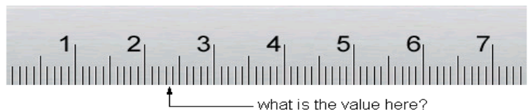
Fig A1: Standard ruler has a maximum uncertainty of \pm 0.5 \text{ mm} . So, the value and its error is 23.5 \pm 0.5 \text{ mm} .
