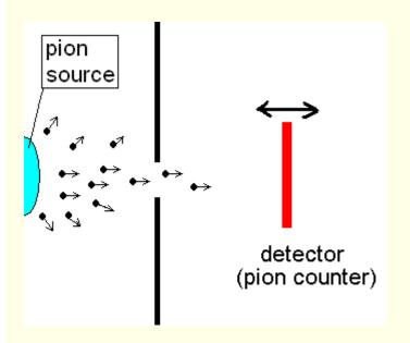
A counter is moved along the pion beam and measured the number of pions at various distances.
