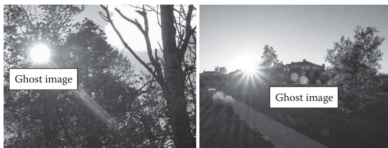
FIGURE 4.41 Two examples of ghost images caused by unwanted focusing of scattering of rays.
