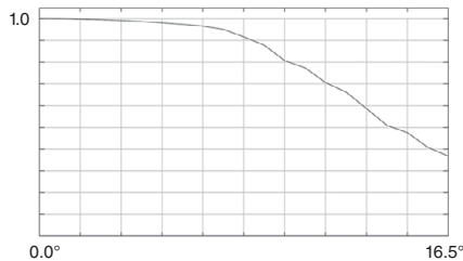
Figure 8.10 Relative illumination of the Petzval portrait objective lens.
