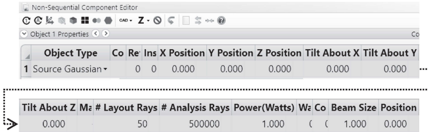
FIGURE 8.8 A Non-Sequential Component Editor box containing a collimated Source Gaussian beam.
