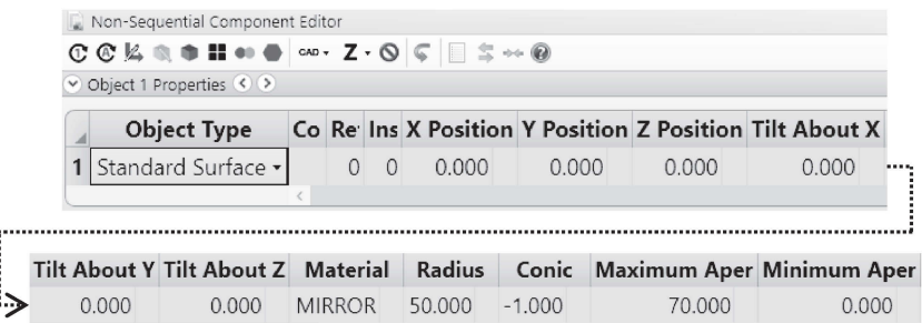
FIGURE 8.5 A Non-Sequential Component Editor box containing a parabola-shaped Standard Surface .
