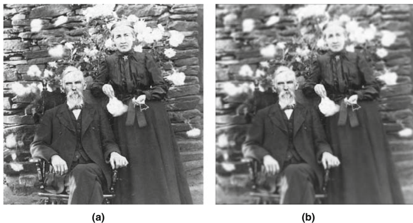
Figure 11.15 (a) Original photograph. (b) Image formed by Section 2.5 cemented doublet showing the effect of astigmatism.
