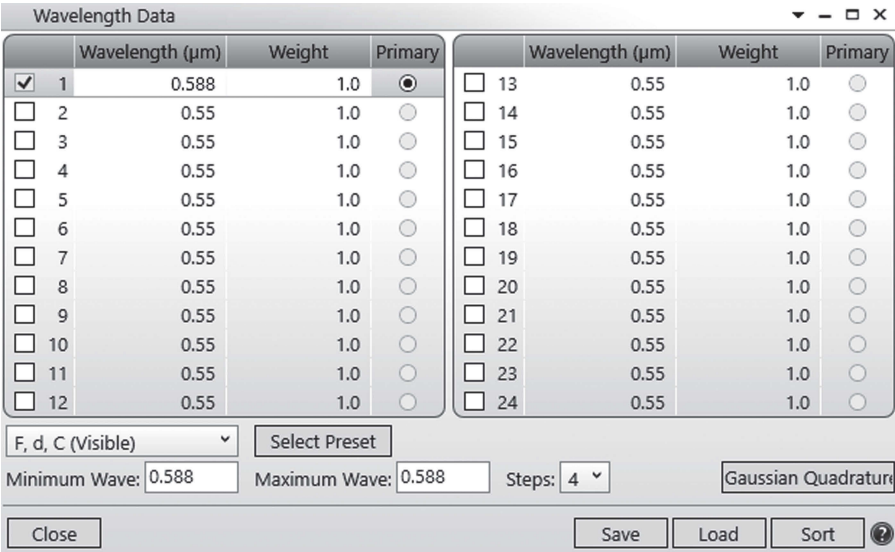
FIGURE 6.2 Select wavelength and weight in Setup/Wavelengths/Wavelength Data box.
