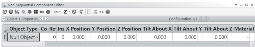
FIGURE 8.2 A Non-Sequential Component Editor box that contains only one row.
