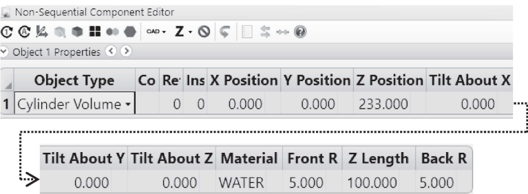
FIGURE 8.6 A Non-Sequential Component Editor box containing a Cylinder Volume filled with water.
