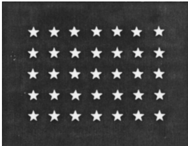
Figure 3.5. Extended source as a collection of point sources.
