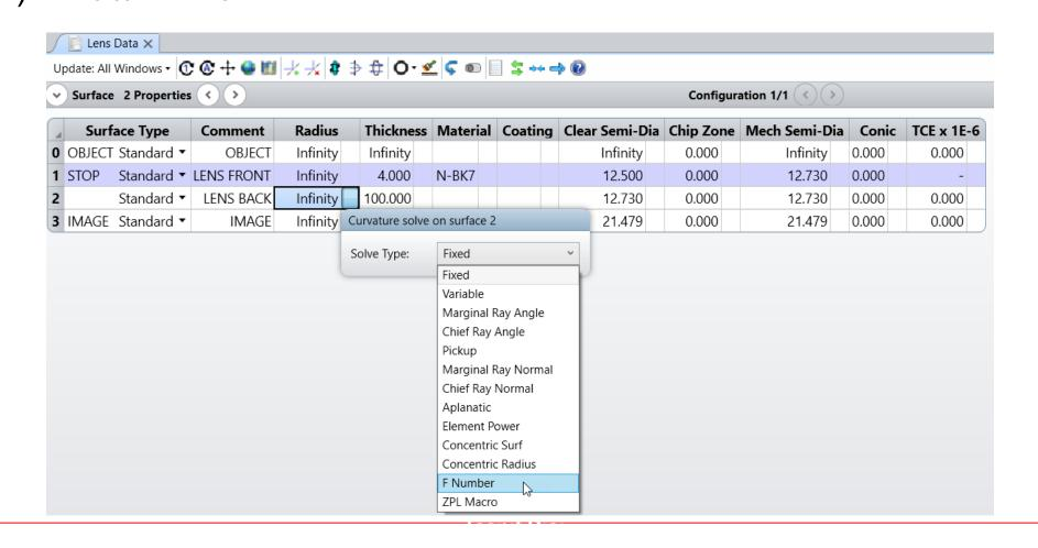
Set Radius of first surface, center thickness and distance between image plane and last surface of the lens are variables.
