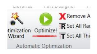
Local optimization uses gradient search to find the nearest merit function minimum and moves "downhill." Global optimization attempts to find the global minimum by allowing both uphill and downhill movement in the merit function.
