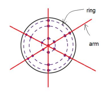
Gaussian quadrature (GQ) sampling uses a very small number of skew rays at very specific pupil coordinates and weightings. GQ sampling returns a mathematically exact integral of the pupil with fewer rays and provides higher sampling near the edge. GQ is the fastest sampling for the majority of cases.
