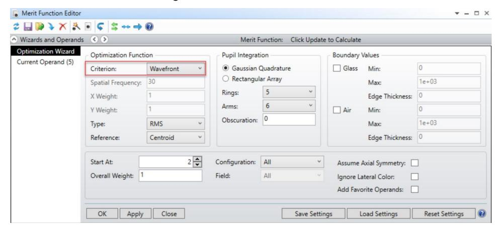
Note that we can build a default Merit Function to minimize wavefront error, spot radius (and X, Y individually) or angular error as a radius or as x and y separately. In this case, we will choose Wavefront, and use 5 rings in the Gaussian Quadrature algorithm because we want a well-corrected system.
