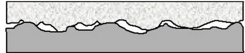
(b) Ceramic asperities indent the metal surface that yields plastically under large local stress.
