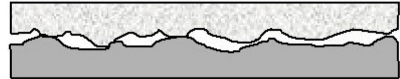
(a) Hard ceramic and ductile metal surfaces come into contact at asperity tips.
