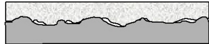
(c) Deformation continues primarily in the metal, leading to a filling of interfacial voids.
