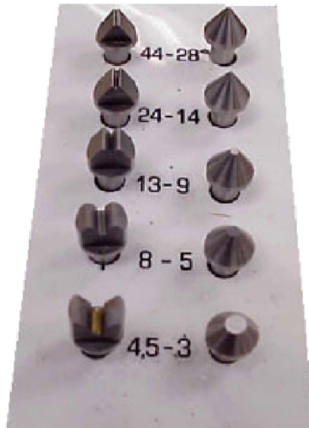
Screw thread micrometer with interchangeable spindle and anvil
