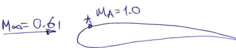
By definition, the critical Mach number is that free-stream Mach number at which sonic flow is first encountered on the airfoil.
