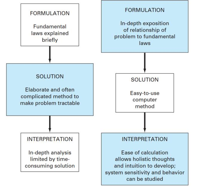
The three phases of engineering problem solving in(a) the precomputer and(b) the computer era.
