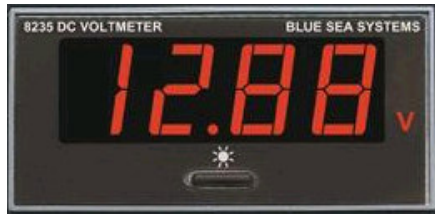
Figure 5: A digital voltmeter having a maximum uncertainty of \pm 0.005 V for this reading.
