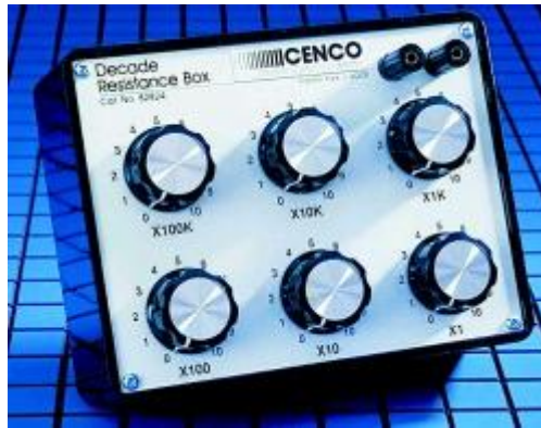
Figure 1.6: A resistance decade box.
