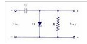
Set-up the circuit of Figure 1 in the lab sheet. Set the input voltage signal to a sinusoid with 1kHz frequency and 12V peak-to-peak amplitude with R=1k $\Omega$ (or set the frequency,V peak-to-peak and resistance). Obtain and plot the input and output voltage waveforms.
