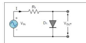
Set-up the circuit of Figure 1 in the lab sheet. Set the input voltage signal to a sinusoid with 1kHz frequency and 12V peak-to-peak amplitude with  $R=1k\Omega$  (or set the frequency, V peak-to-peak and resistance). Obtain and plot the input and output voltage waveforms.
