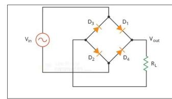
Set-up the circuit of Figure 1 in the lab sheet. Set the input voltage signal to a sinusoid with 1kHz frequency and 12V peak-to-peak amplitude with  $R=1k\Omega$  (or set the frequency, V peak-to-peak and resistance). Obtain and plot the input and output voltage waveforms.
