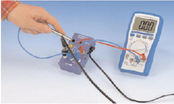
Figure 6: Connection of the electrometer amplifier
