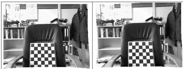
Fig. 2: After rectification operation some useless areas appear on both left and right images
